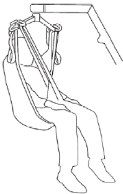
Properly connected sling to cradle
