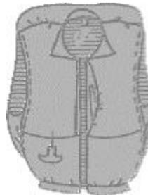
Special use PFDs include work vests, deck suits, and hybrids for restricted use. Hybrid vests contain some internal buoyancy and are inflatable to provide additional flotation.
