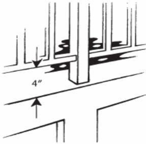
In addition, if an above-ground pool has a barrier on the top of the pool the **maximum vertical clearance between the top of the pool and bottom of the barrier should not exceed 4 inches.**
